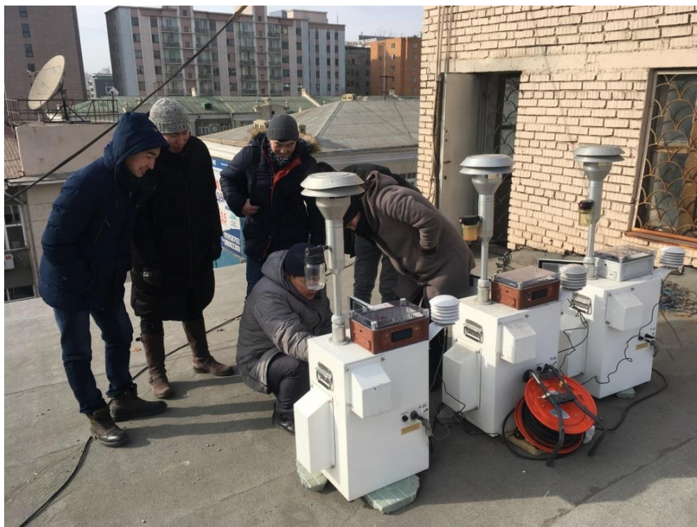
Figure 3.4: Measurement training at partisol gravimetric PM samplers on the roof of the NAMEM building (Photo: G. Baumbach 2019)
